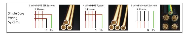
In a MIMS 3 wire ESR multiphase wiring system, the combined cross sectional area of the copper sheath of three single core Pyrotenax 3E MIMS cables is > 100% of the active conductor for sizes up to 400 mm<sup>2</sup>.
