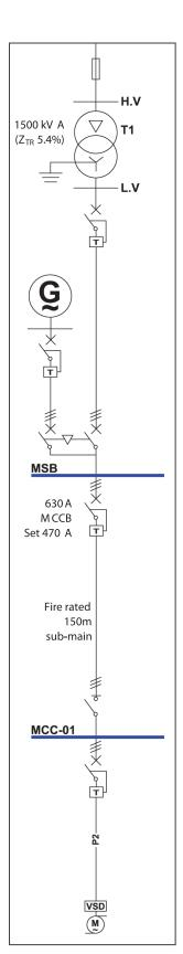
PowerCad-5™ electrical engineering design software provides the platform for engineers to rapidly model LV distribution networks. Once modelled "what if" scenarios as to cable wiring systems, protective device options switchboard configurations can be tested with the software dynamically designing and checking each scenario for compliance with AS/NZS3000:2007.
